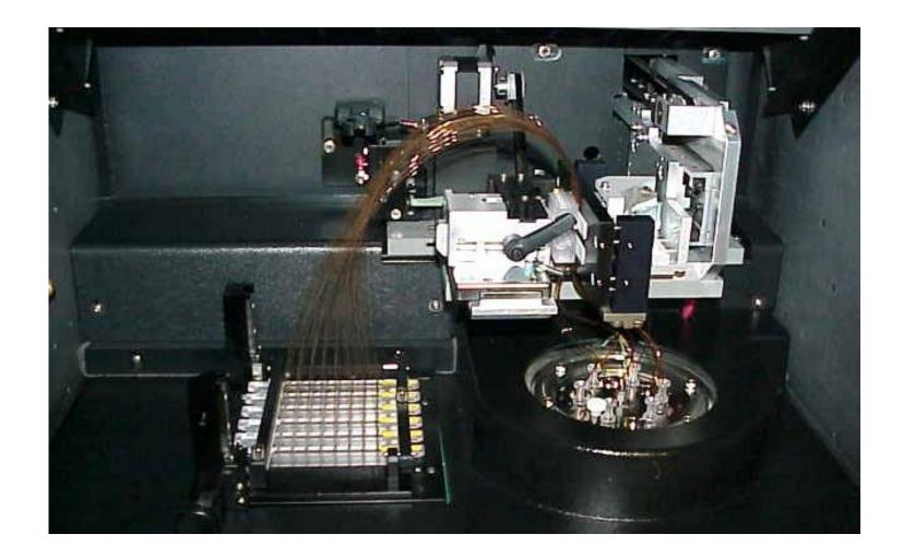
The brown wire-like loops are the 96 individual capillary tubes. They are made of glass and coated with brown plastic. The samples are loaded from below this level on the left side and the DNA is electrophoresed towards the right. The matrix is injected into the tubes after each run and it travels from right to left when filling the tubes.
